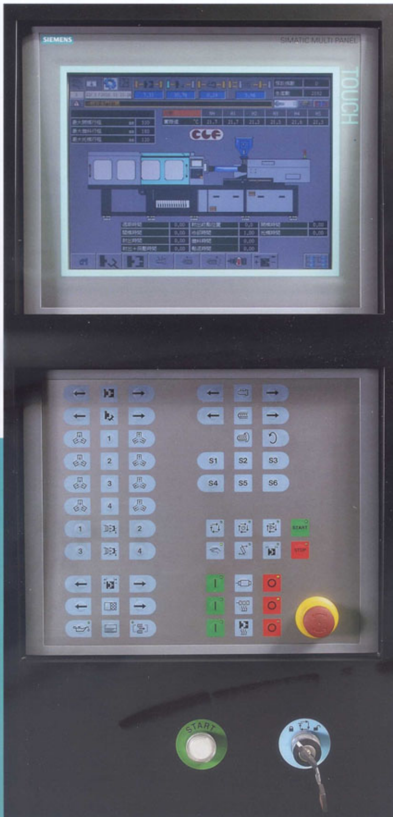
Mold open/close setting display
