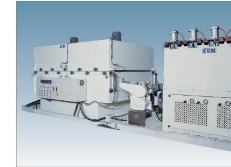
Take Off Unit & Drying Oven
