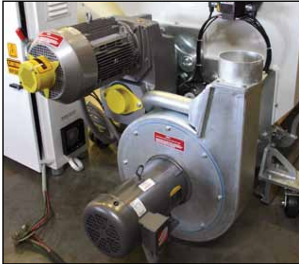
Safe manual Reverse Interlocked Access And Sound suppression Blower.
