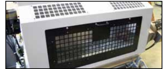
Cutting Chamber Access Door
